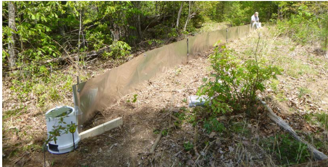
A camera trap drift fence placed in Cherokee County for detecting northern pinesnakes. Modified trail cameras are suspended in the buckets at the ends of the fence. NCWRC Conservation Technician, David Woody, finishes securing one of the camera trap buckets to the fence. (Photo: NCWRC)
