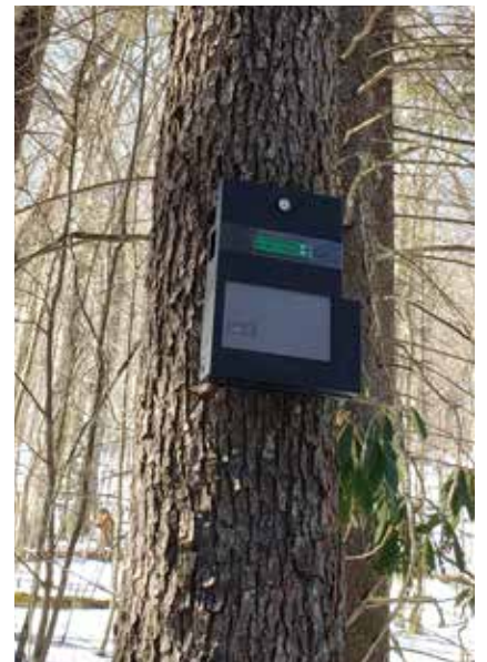
A Songmeter recording unit deployed in northern saw-whet owl habitat. (Christine Kelly)
