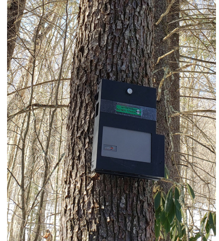
A Songmeter recording unit deployed in northern saw-whet owl habitat. (Christine Kelly)
