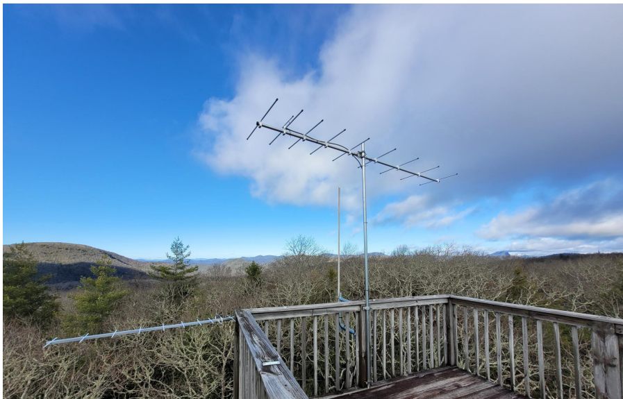
A “dual mode” Motus station. The large yagi antenna (right) is tuned to 166.380 MHz while the smaller yagi antenna (left) is tuned to 434 MHz. (Christine Kelly)
