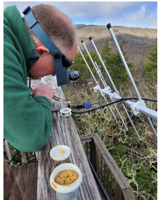
Clockwise from top left: The NCWRC is on the Motus map. Motus station at the Mountain Retreat and Learning Center on Little Scaly Mountain is circled in red (Motus.org). Kendrick Weeks, Western Wildlife Diversity Program Supervisor solders a connector to a coaxial cable. (Christine Kelly). An infographic from Birds Canada about the Motus Wildlife Tracking System (Motus.org)
