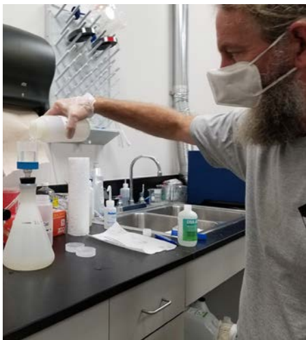
Wildlife Diversity technician, Reed Rossell, in the lab processing river water samples with a vacuum flask, special filters to trap DNA, and an electric pump. (Lori Williams)
