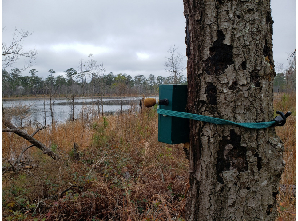
Automated audio data logger, AKA "froglogger" (Photo: Jeff Hall)
