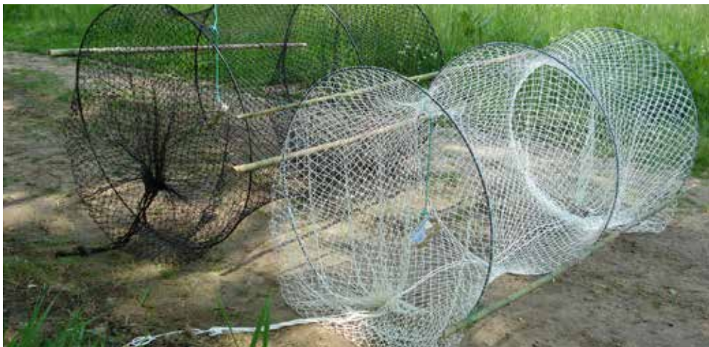
Example of hoop traps used for capturing aquatic turtles (Photo: Sam McCoy)
