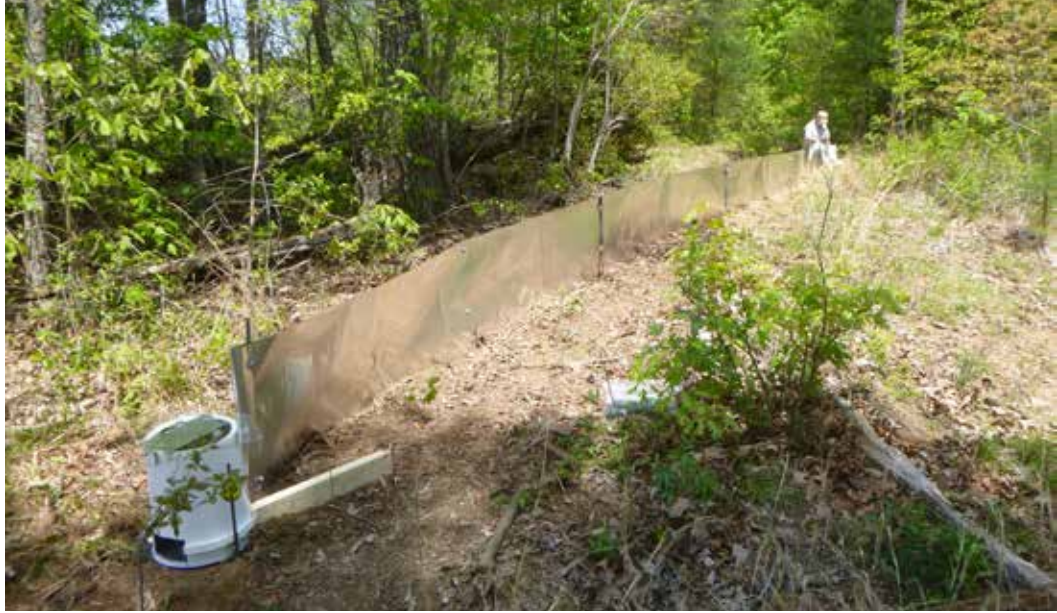
A camera trap drift fence placed in Cherokee County for detecting northern pinesnakes. Modified trail cameras are suspended in the buckets at the ends of the fence. NCWRC Conservation Technician, David Woody, finishes securing one of the camera trap buckets to the fence. (Photo: NCWRC)
