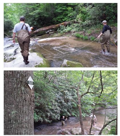
N.C. State University researchers scanning for PIT-tagged trout via a floating antenna (Fixed-antenna arrays were stationed at upper and lower ends of each study reach.) (Photos: Jacob Rash)
