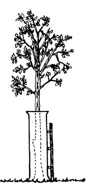
Fig. 14. Tubex® tree shelters are a new individual seedling protector designed for deciduous tree seedlings.
