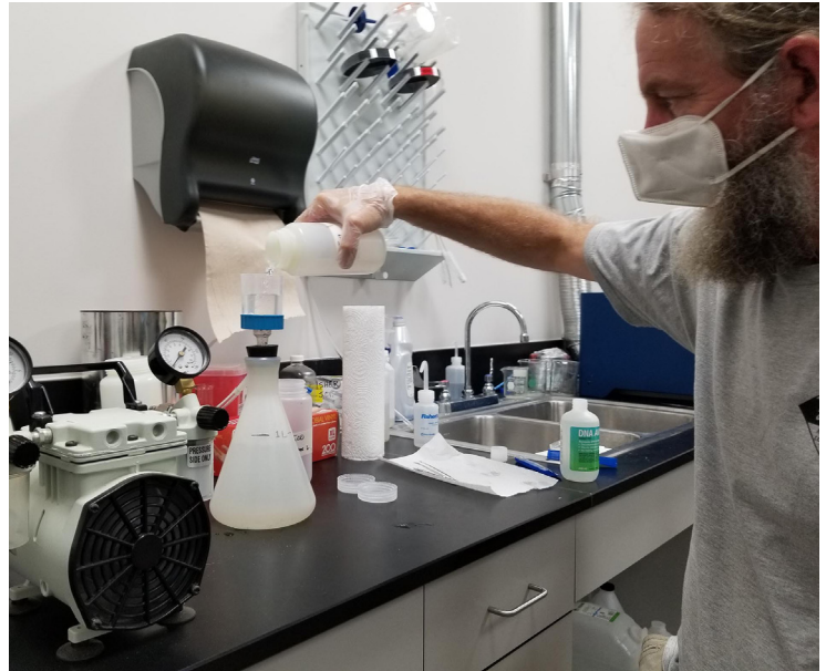
Wildlife Diversity technician, Reed Rossell, using an electric pump and vacuum flask to filter water samples in the lab, 2021 (Lori Williams)
