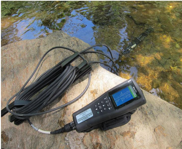
A water quality meter in use at a study site, measuring parameters such as temperature, pH, conductivity, dissolved oxygen, turbidity, salinity, and total dissolved solids. (Photo Lori Williams)
