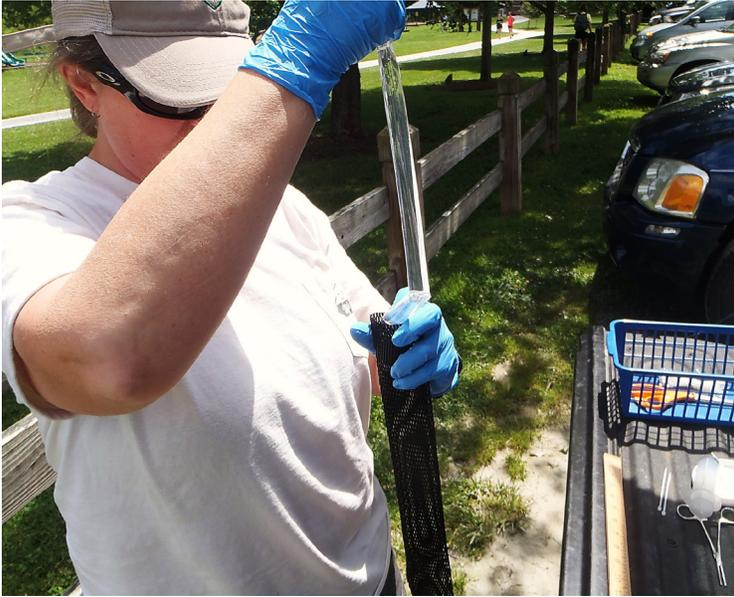
Wildlife Diversity staff inserts dialysis tubing filled with deionized water into a protective sleeve to be installed at eastern hellbender habitats to determine agrochemical and heavy metal presence in rivers; the membrane of the dialysis tubing mimics a hellbender's semi-permeable skin. (Photo John Groves)
