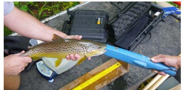
Stocked Brown Trout have a small piece of metal, also known as a “tag,” embedded in the cheek. The “tag wand” acts as a metal detector. Using this technique NCWRC biologists can determine if the fish is stocked or wild, how old the fish is, and how fast it is growing. (Photo: Chris Wood)
