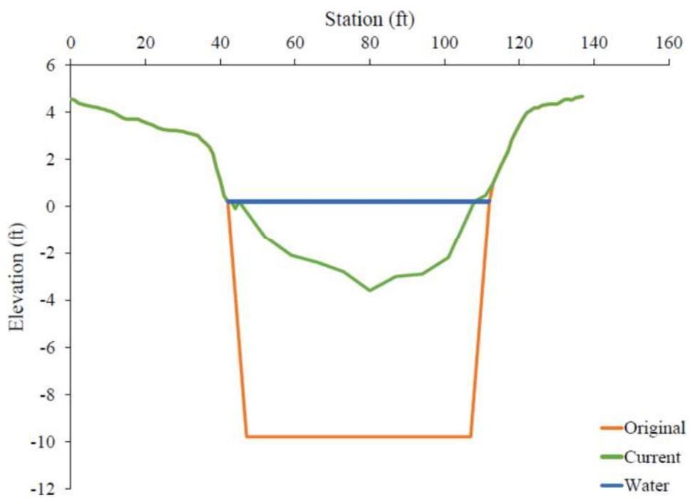
FIGURE 8. Cross-section view of depth measurements of Outfall Canal collected by Dr. Randall Etheridge, East Carolina University. Current canal depth is the green line. Red lines depict the original depths at time of canal excavation. Water level is demonstrated by blue line.
