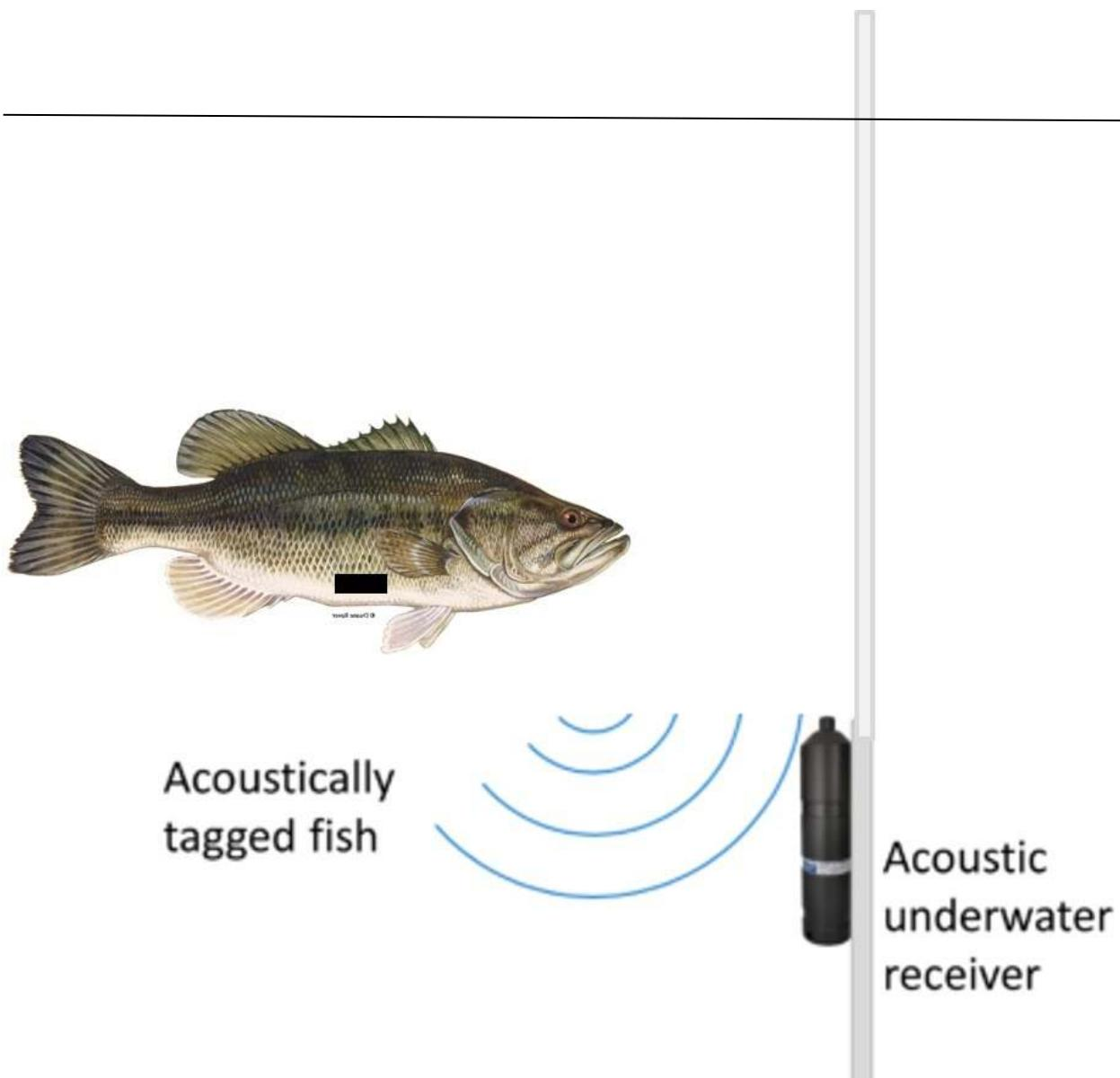
FIGURE 2. Illustration of acoustically tagged Largemouth Bass detected at an underwater passive acoustic receiver station at Lake Mattamuskeet. Illustration is not to scale.
