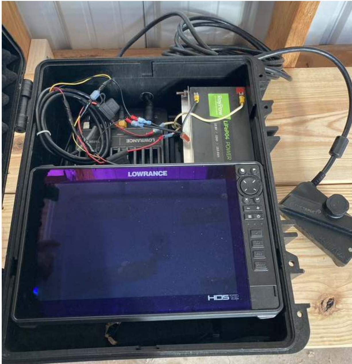
Figure 1. Lowrance ActiveTarget sonar processing unit, Lowrance HDS-12 live chartplotter, and lithium-ion 12V x 12Ah battery mounted within a waterproof case. The ActiveTarget transducer is visible to the right of the case and affixed to the transom of the boat using EMT conduit and a trolling motor mount when in use.
