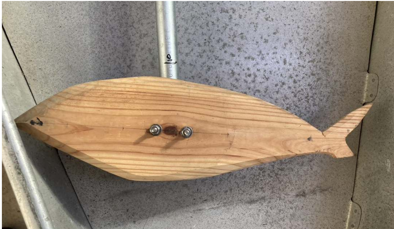
Figure 3. Known-length (500-mm TL) target. Target was constructed of southern yellow pine to the approximate proportions described for American Shad by Menhinick (1991) and mounted on a 3-m length of EMT conduit.
