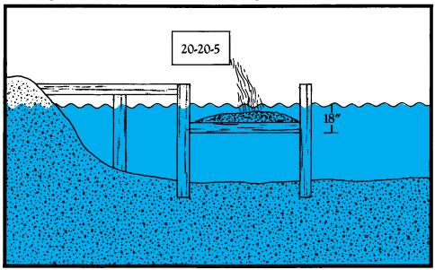
Figure 9. Platform for dispersion of granular fertilizer.
