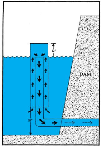
Figure 2. Drainpipe incorporating a device for drawing water from the bottom of the pond.
